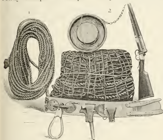
1, LIFE ROPE; 2, LIFE RIFLE LINE; AND 3, JUMPING NET; 4, BELT WITH SNAP AND TOOLS.
